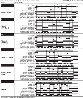
XIn case of F, F1 output operation mode, setting time should be over 100ms.
